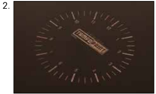
Fig.: bad laser engraving
