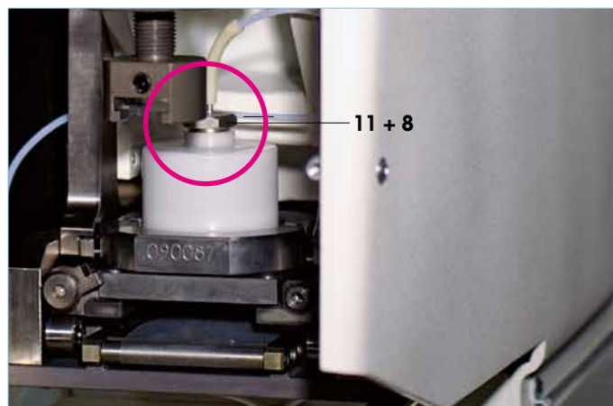
III.: Discharge hose (8) is mounted to the ink/doctoring cup (12) by means of sealing plug (11)
