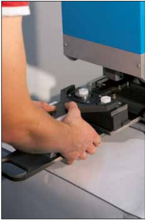
Installation/removal of printing unit using special gripping tongs and assembly table
