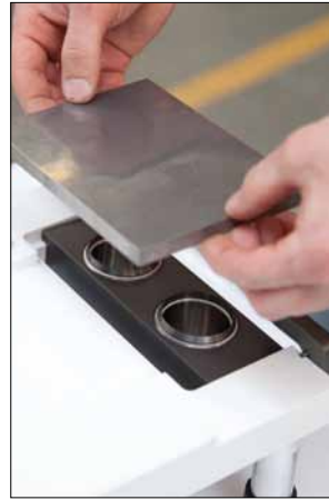
Ink/doctoring cup bridge with 2x Ø 42 mm ink/doctoring cups
