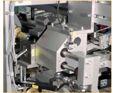
Fig: Infeed station as well as a special jig carrier system with clamping mechanism
